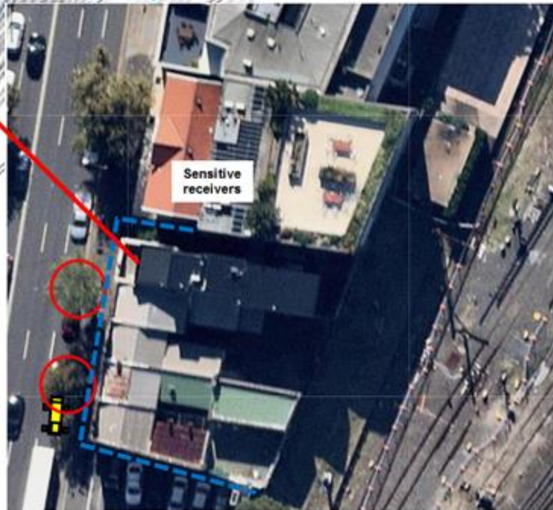
○ - Trees to be removed 🚧 Location of chipper - - - Hoarding
