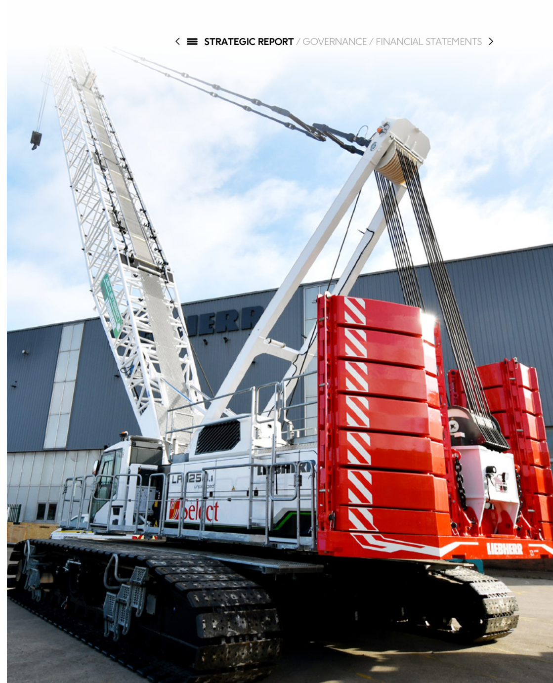
Image: Electric crawler crane – Liebherr LR1250.1 250t lattice jib crawler crane
